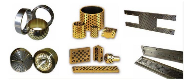
The **INSERTS IN GRAPHITE** are distributed over 20-30% of the running surface, creating an anti-friction thin film that will remain during the rest and is under heavy loads. On request could may be applied a film of 20 um of composition similar to that of the insert to facilitate the early movements and avoid a damaging blow to departure (stick-slip).
