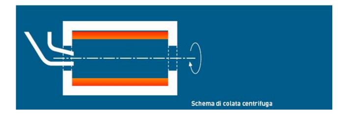
The combined effects of centrifugal force and the progressive solidification under pressure metallostatic very high, leading to a fine grain structure, free of porosity and hence higher mechanical properties compared to castings obtained by traditional methods.
